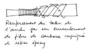
To prevent the resin dripping, I wind Teflon tape around the binding. This is long, delicate and messy, but it makes reeds that work.
