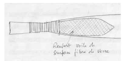
Option 3: I stick to the center of each blade a backbone made of fibreglass or carbon impregnated with epoxy or glued with cyano. The edge goes from the wrapping of the reed up to 1 cm from the tip.
