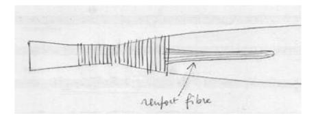
All these options have the same function: the winding of fibre on the heel (option 1) raises the pitch, and reduces the scope of freedom of the reed. The addition of a backbone (option 3) darkens the sound. Bonding of cloth to the surface (option 2) combines the two above effects. You have to decide which to choose based on the observed behavior of the reed (timbre, pitch, field of freedom).
